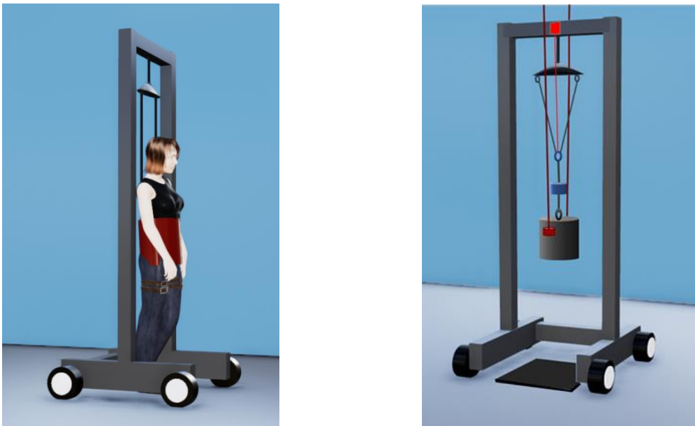
Figure 1: Left: Subject in a (partial) Weight Support system, Right: Concept of the test setup
