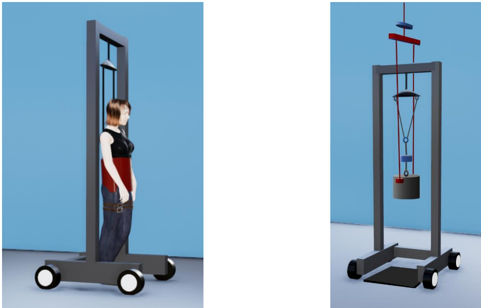
Figure 1: Left: Subject in a (partial) Weight Support system, Right: Concept of the test setup
