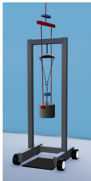
Figure 2: Structure of the test arrangement –the force sensors shown in blue, the crane in red
