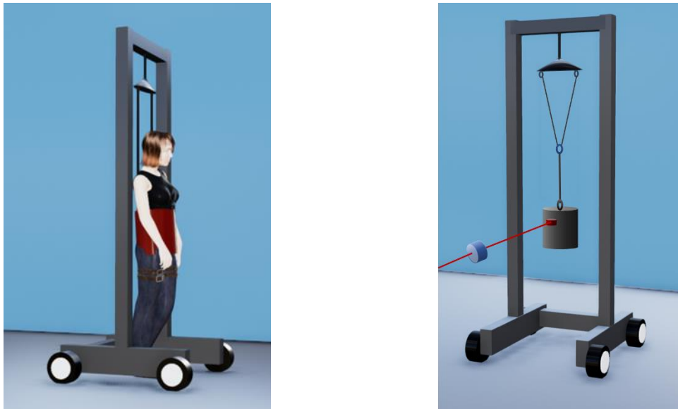
Figure 1: Left: example of use situation, with movement direction (A), the lateral roll (B) and the anterior posterior pitch (C); Right: concept of testing setup
