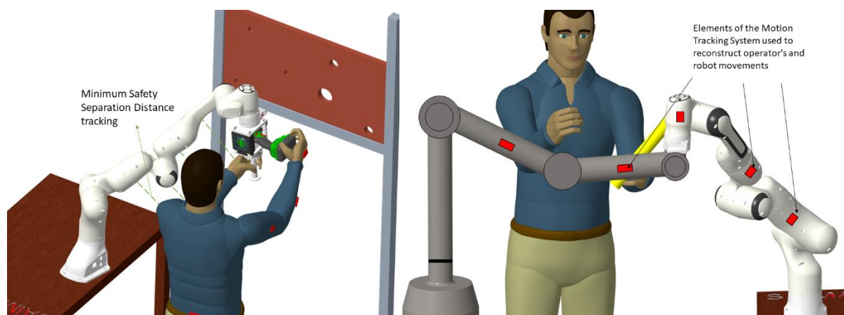
Figure 1: Example of minimum distance between robot and operator in a hand guiding robot application (left) and MSD-skill test setup (right)
