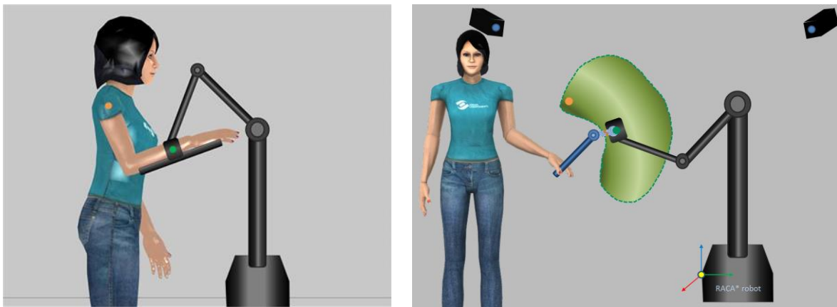
Figure 1: Example of ROM* related RACA robot* in a rehabilitation application (left) and LRM*-skill test setup (right)
