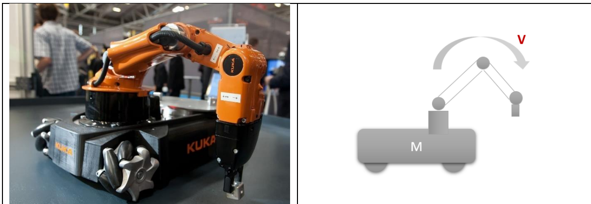
Figure 2: Example of a robot arm on a mobile platform moving in such a way that it may cause the base to become unstable
