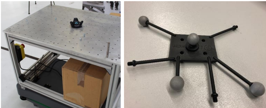
Figure 3: A rigid body marker hold on a mobile platform (left) and a marker set on a support for rigid body tracking (right)
