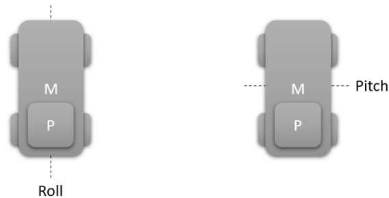
Figure 1 Roll and pitch rotation axis. M is a mobile platform and P is a payload
